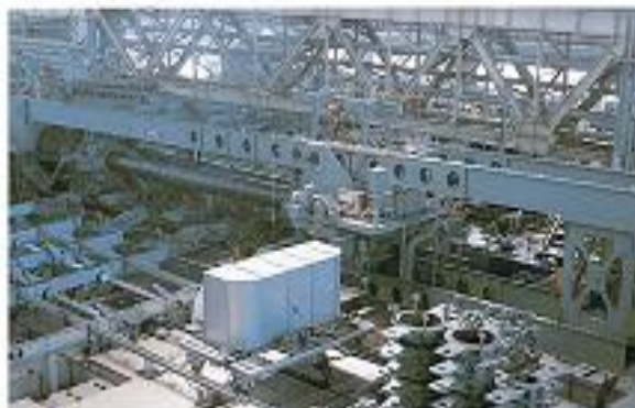
UOE大径鋼管水圧試験機 Hydrostatic Pipe Tester (for UOE large dia. pipe)
